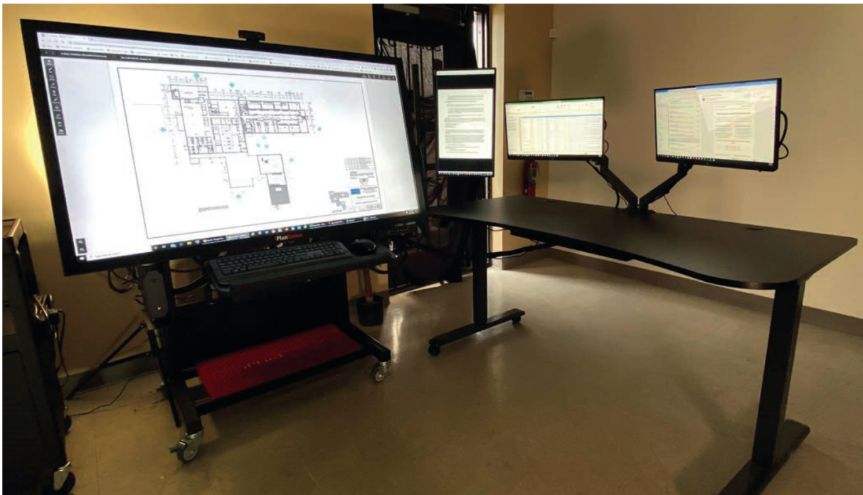
Figure 1-13. This wide-format display table has a large touchscreen monitor and is equipped with three smaller monitors for additional display.
